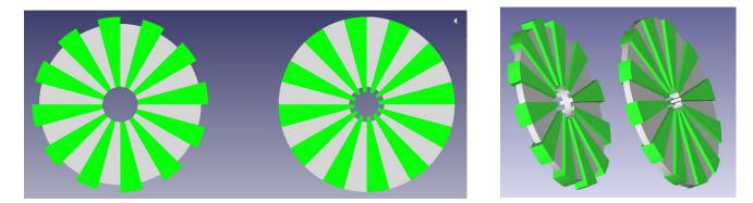
The "stack" comprises two alternating disk designs that have matching raised segments and are made of a conducting material. In this example each segment is 15 degrees wide with 15 degree gaps. But so long as the gaps are no wider than the raised segments other angles can be used. One disc type has the segments projected outside the perimeter, where they engage in slots in a surrounding tube. The other type has the segments projected towards the centre, where they engage in splines on a
